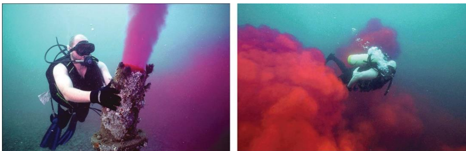
FIGURE 3. Rhodamine dye tests undertaken at the Perth Seawater Desalination Plant. 84
